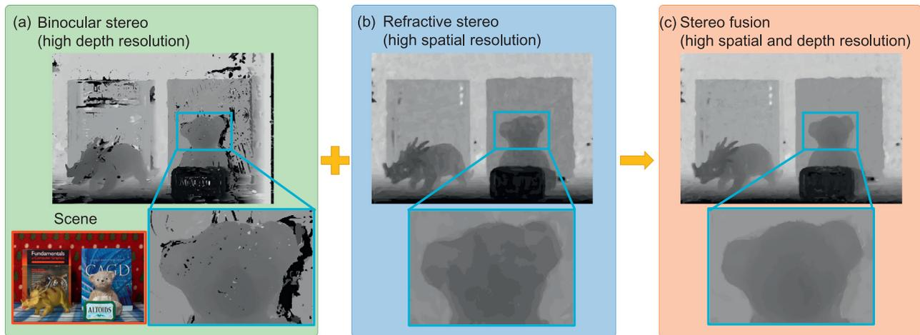
**Fig. 1.** (a) Binocular stereo detects depth accurately, whereas it suffers from spatial artifacts caused by occlusions and featureless regions. (b) Refractive stereo improves the spatial resolution with fewer artifacts, but its depth resolution is coarse with fewer steps. (c) Our stereo fusion significantly improves both spatial and depth resolution by combining these two heterogeneous stereo methods.
