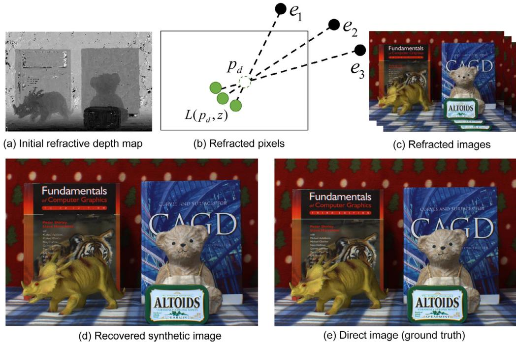
**Fig. 7.** (a) Shows an initial depth map. (b) shows the computed positions of refracted pixels corresponding to the three essential points using the depth estimates (a). We recover a synthetic direct image (d) by computing the arithmetic mean of the corresponding refracted pixel colors (b) on the refracted images (c). (d) and (e) compare the synthetic image with a ground truth image that was captured while the medium was detached.
