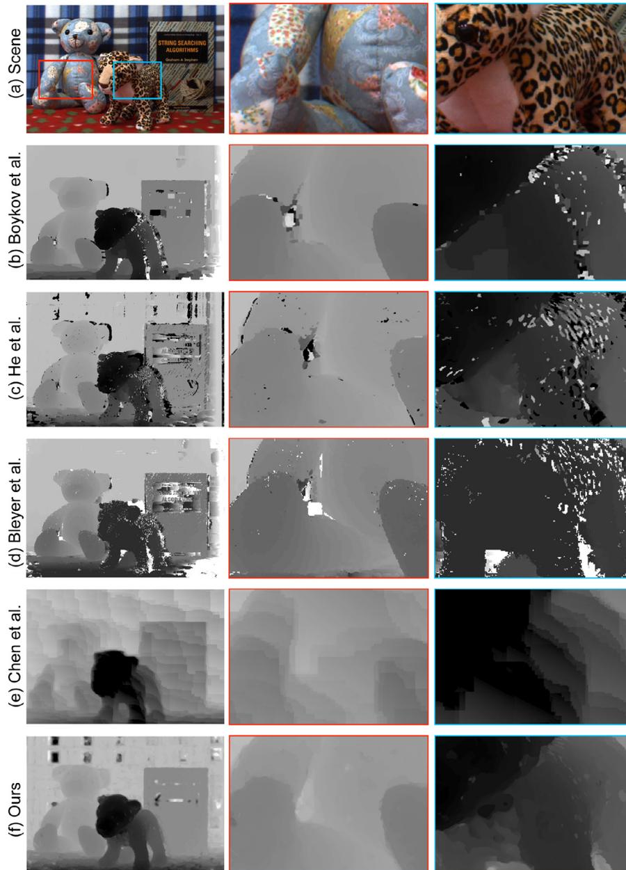
**Fig. 14.** Depth maps of a scene (a) are computed by five different methods. (b) and (c) show depth maps produced by global [38] and local binocular stereo [32] methods. (d) shows the depth maps obtained by a patchmatch-based binocular stereo method [39]. (e) presents depth maps produced by a refractive stereo method [10]. Our method (f) estimates depth accurately without suffering from severe artifacts.
