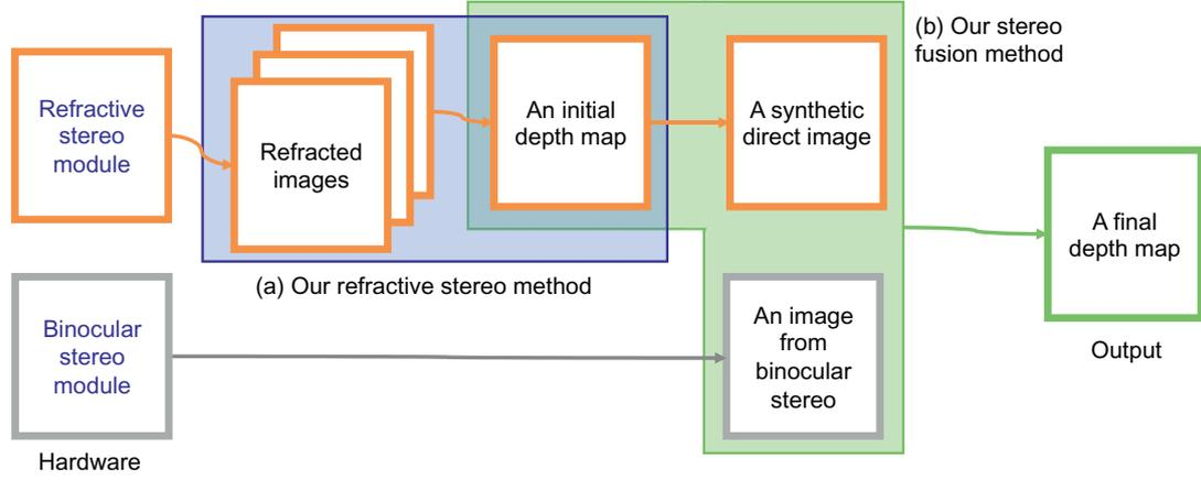
**Fig. 6.** Schematic diagram of our stereo fusion method. (a) Our refractive stereo method estimates an intermediate depth map from refractive stereo. (b) Our stereo fusion method reconstructs a final depth map from a pair of an image from binocular stereo and a synthetic direct image obtained using the intermediate depth map.
