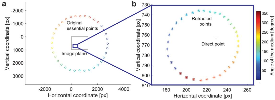
**Fig. 4.** (a) Presents the calibrated results of 36 essential points measured by Baek and Kim's method [12]. (b) shows the locations of 36 refracted points from a direct point in the coordinates of (763,229) at a distance of 40 cm. This figure shows that the direct point is refracted to 36 different positions depending on the medium orientation.
