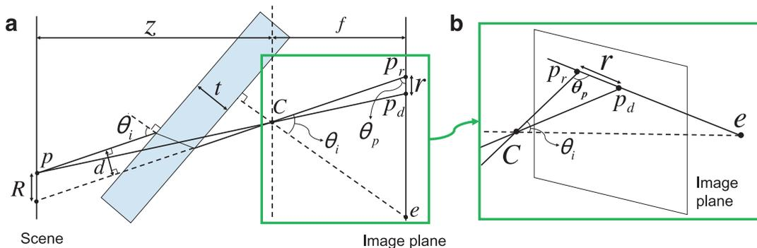
Fig. 2. (a) Cross-section view of the light path in refractive stereo. (b) Close-up view of refractive light transport in 3D.
