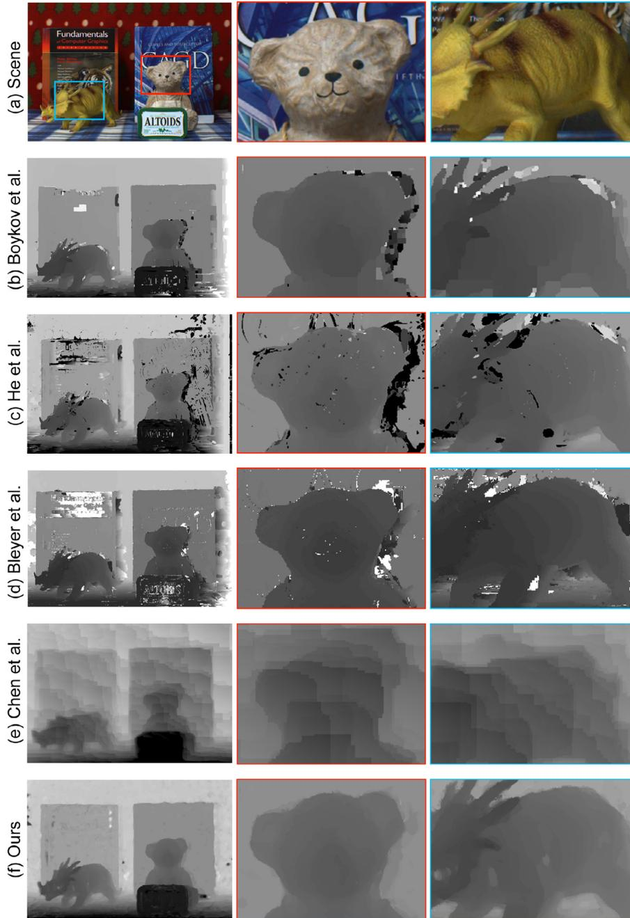
**Fig. 13.** Depth maps of a scene (a) are computed by five different methods. (b) and (c) show depth maps produced by global [38] and local binocular stereo [32] methods. (d) shows the depth maps obtained by a patchmatch-based binocular stereo method [39]. (e) presents depth maps produced by a refractive stereo method [10]. Our method (f) estimates depth accurately without suffering from severe artifacts.
