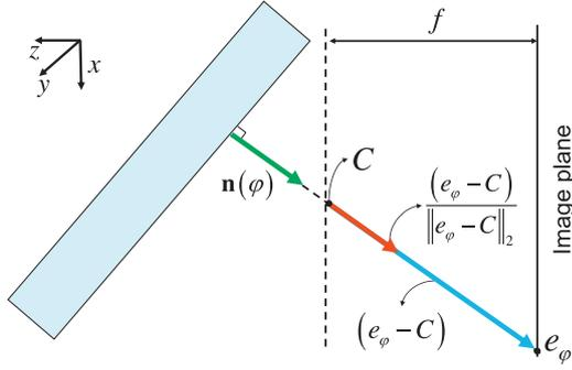
**Fig. 5.** For angle  $\varphi$  of the medium, essential point  $e_\varphi$  is formed as an intersection point in the image plane on a line that passes through the center of optics  $C$ . The unit normal vector of the medium  $\mathbf{n}(\varphi)$  is on the same line.
