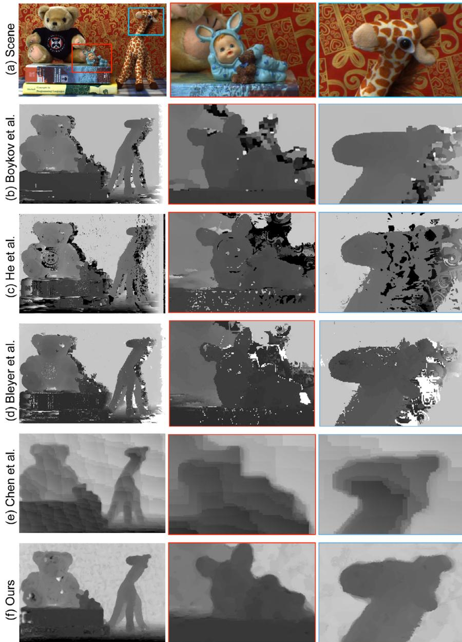
**Fig. 15.** Depth maps of a scene (a) are computed by five different methods. (b) and (c) show depth maps produced by global [38] and local binocular stereo [32] methods. (d) shows the depth maps obtained by a patchmatch-based binocular stereo method [39]. (e) presents depth maps produced by a refractive stereo method [10]. Our method (f) estimates depth accurately without suffering from severe artifacts.
