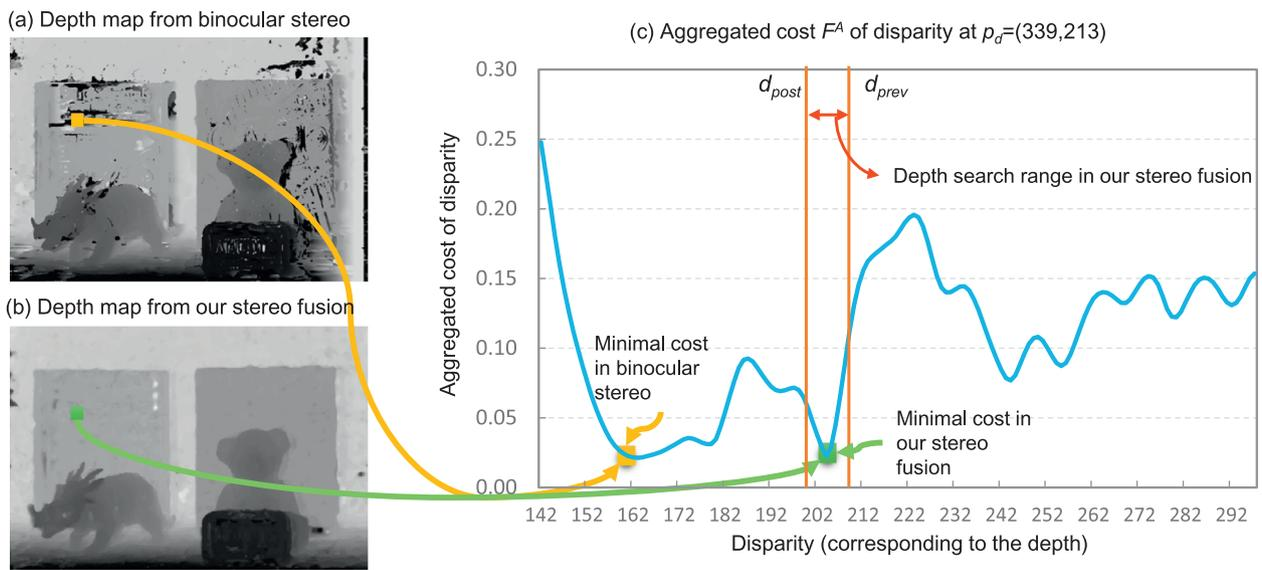
**Fig. 10.** The binocular depth map (a) includes artifacts due to false matching caused by occlusions, featureless regions and repeated patterns. Using the intermediate refractive depth map (b), we can limit the search range of a corresponding point  $p_d$  between  $d_{post}$  and  $d_{prev}$  for instance. This significantly reduces false matching frequency in estimating depth.
