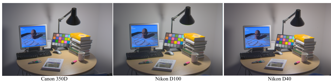
Figure 6: An HDR desk scene is characterized with our method for three different digital cameras. Even though they are taken in slightly different perspective and angles, there are only very minor color differences between the images.
