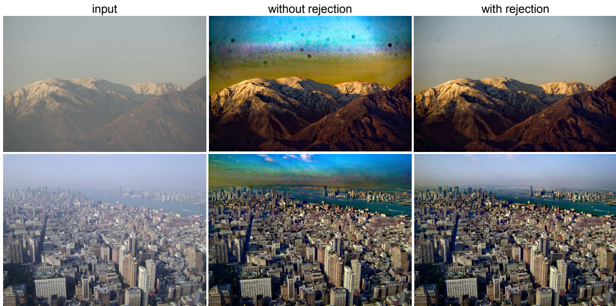
Figure 5.6: Validation of our narrow angle outlier rejection method described in Section 4.1.3. In the second column, the distant region represented as sky has an infinite depth, and hence our transmission estimation stage estimates its transmission as being close to zero, which yields overly saturated results. We obtained consistent results by our outlier rejection stage, as shown in the third column.
