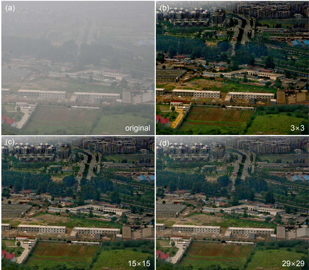
Figure 5.5: Comparisons to show the influence of a patch size in estimating transmission. (a) The original canon image. (b) The dehazed image with a patch size of 3 \times 3 where severe color clamping happens. (c) The dehazed image with a patch size of 15 \times 15 , where the patch size is our choice for all results. (d) The dehazed image with a patch size of 29 \times 29 in which the airlight in distant regions is underestimated.
