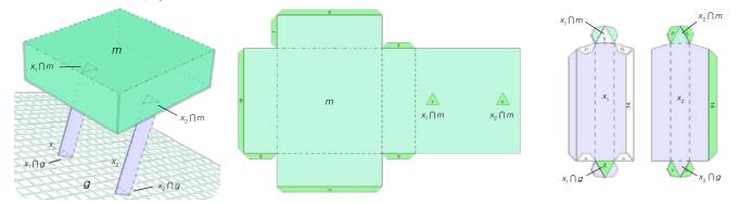
Fig. 9. In (a), a basic example model with two added supports, denoted  $m \cup x_1 \cup x_2$ , is shown standing on the ground plane g. (b) shows the unfolded model m with added assembly guides, while (c) shows both sides of the unfolded support  $x_1$ .
