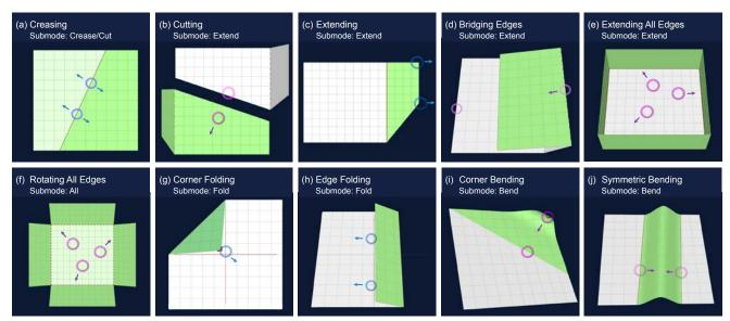
Fig. 3. Representative 3D modeling tools: (a) creasing a sheet of paper, (b) cutting along an edge, (c) extending along an edge of a face, (d) bridging edges of two faces, (e) extending all edges of a face, (f) rotating all faces generated in (e), (g) corner folding, (h) edge folding, (i) corner bending, and (j) symmetric bending. Circles and arrows indicate the position and motion of user touches.
