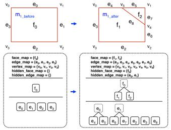
Fig. 5. Overview of the object data structure in our system. The righthand side shows how the data structure is updated when a face of the model is split (e.g., through folding).
